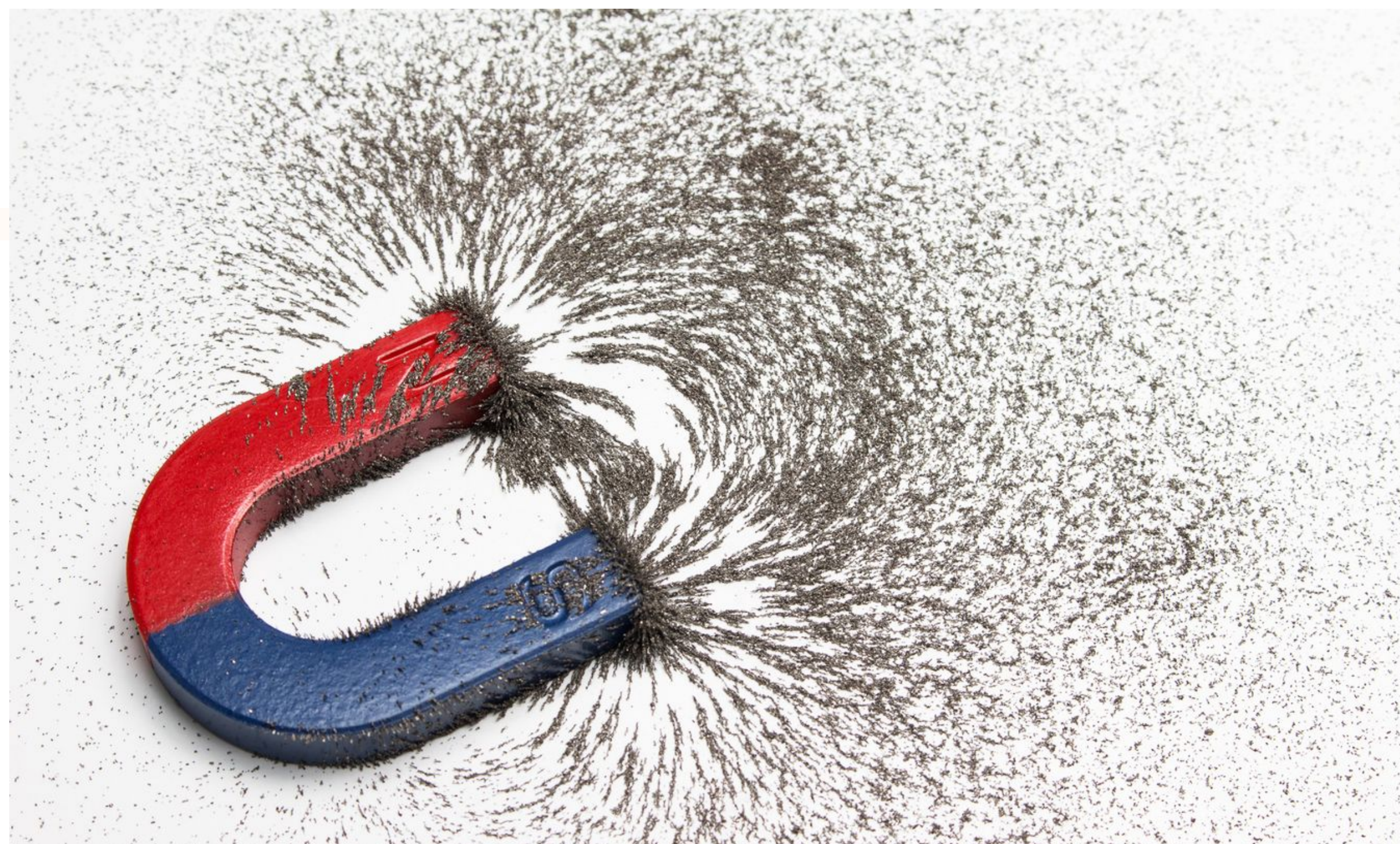
Iron filings visualize magnetic field lines.
